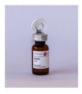
**4)** Open the warm resin vial. (Reclose the vial after use, seal with parafilm.)
