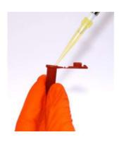
**5)** Pipette 90 μl warm resin and 10 μl crosslinker into the orange Eppendorf. Gently mix to obtain homogeneous solution b.
