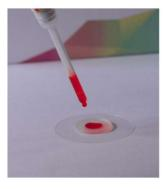
7) Take ~60 µl of the freshly prepared solution from the Eppendorf<sup>c</sup> and add into the mold. Avoid air bubbles.
