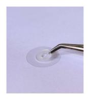
**6)** Place the supplied silicon mold onto the substrate.
